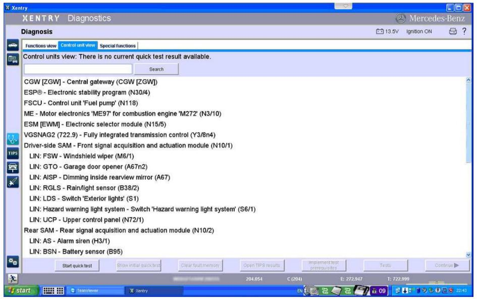
(Control modules are able to be read out in the Control unit view menu)
